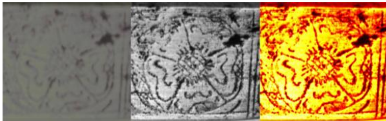
Figure 12: A Tudor rose emblem on a knife comes into view. A careful selection of wavelengths and false colour images will be evaluated to bring clarity. By focusing on small sections it is possible to further enhance the contrast.
