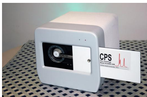
Figure 6: CPS Disc Centrifuge 'UHR'
