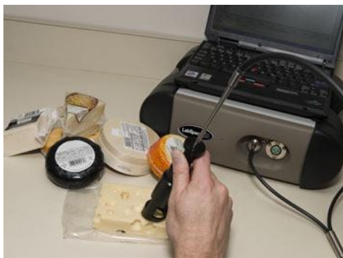
Fig. 1 – The portable ASD LabSpec ® 5000 being used for food analysis
