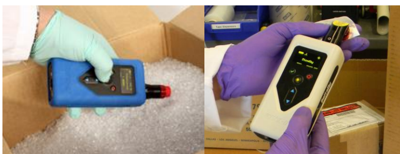
Fig. 3: RAPID-ID (left) and PHARMA-ID (right) handheld Raman spectrometers from DeltaNu
