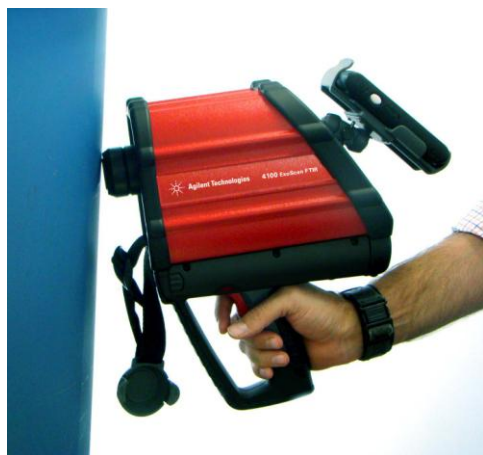
Fig. 2: ExoScan 4100 handheld FTIR
