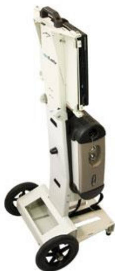
Fig. 3: LabSpec 4 portable NIR spectrometer and GoLab trolley from ASD Inc.
