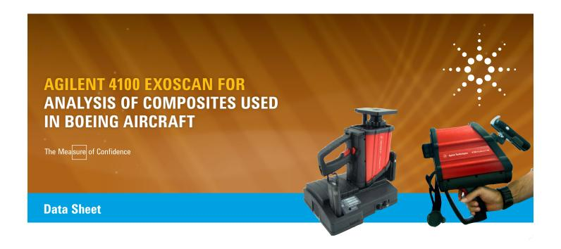
Composites have become popular materials to use in a variety of applications; this includes their usage in the Aerospace and Aviation marketplaces. The 4100 Exoscan FTIR has been shown to be an effective, non-destructive technology for measuring heat exposure in composite materials ("Composite Heat Damage measurement using the handheld Agilent 4100 ExoScan FTIR" by J. Seelenbinder).
