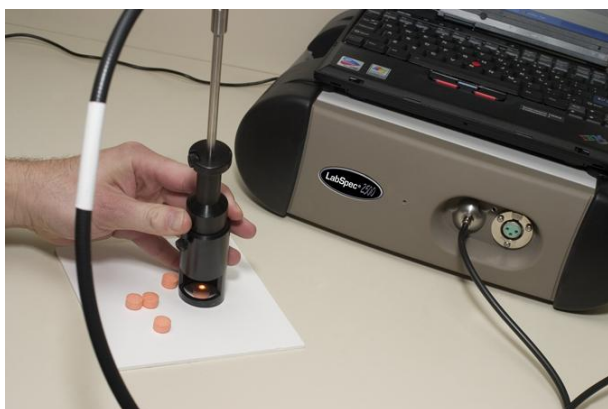
Fig. 2 –ASD LabSpec ® being used for counterfeit drug detection
