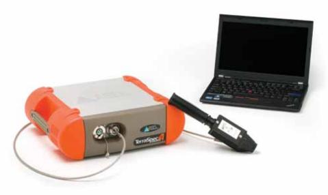
For mining exploration geologists, these improvements translate into faster data capture and improved data quality. The enhancements also allow accurate assessment of low-concentration and low-reflectance minerals, like iron-containing minerals such as serpentines and chlorites, which were previously difficult to measure.
