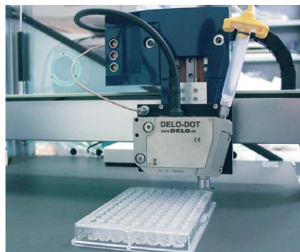
Temperature controlled dispense heads from DELO eject 3 Nanolitre drops and accept viscosities of up to 20.000 mPa's.
