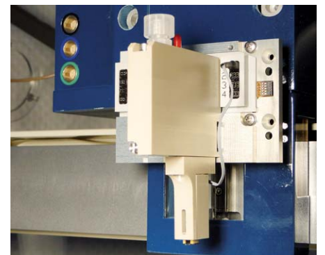
For bulk dispensing of a larger number of smallest drops (from 10 Pikolitres) a reservoir (3 Millilitres) is available for the piezoelectric tips.
