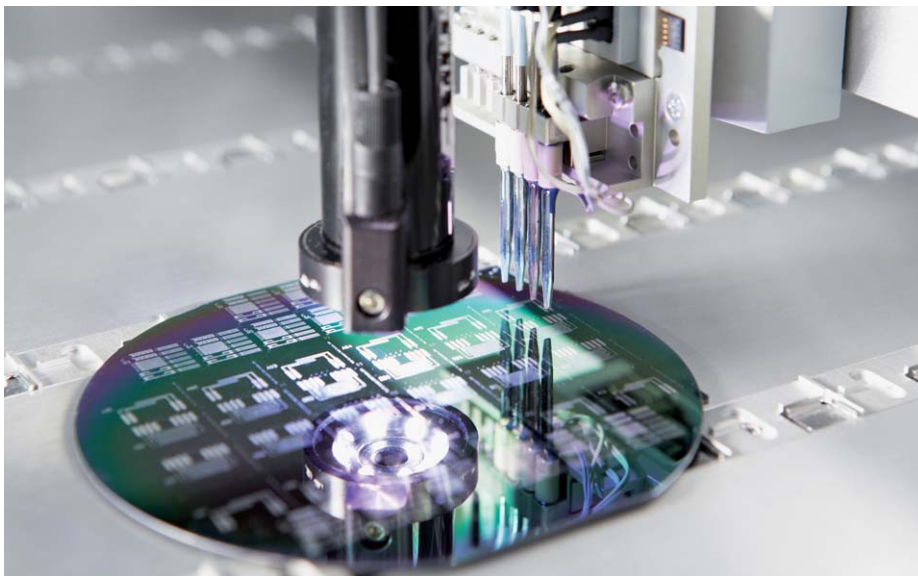
A software extension allows the unlimited definition of dispense positions relative to marker patterns.
