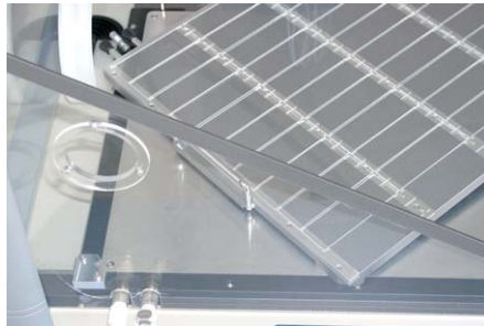
Removable slide tray with underlying chiller plate and temperature sensor
