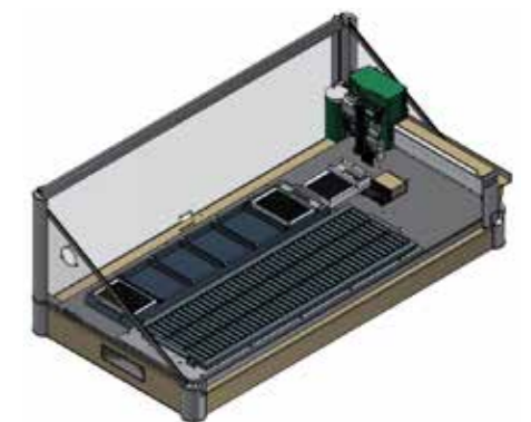
A085-205,242 NP 2.1/E with 6-fold MTP holder and small slide deck for 3 x 41 Zeptosens chips
