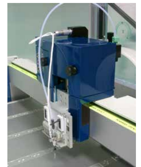
A070-560 Nano-Tip J-H in a Nano-Plotter with extra socket and cable for temperature control (A070-450; in the rubber band, not seen)
