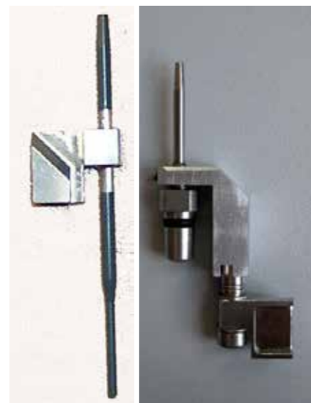
A070-900,901 Dosage capillary ("passive" tip) and adapter for disposable plastic tips. The latter cannot be used together with piezoelectric tips; plastic tips are manually loaded and ejected.
