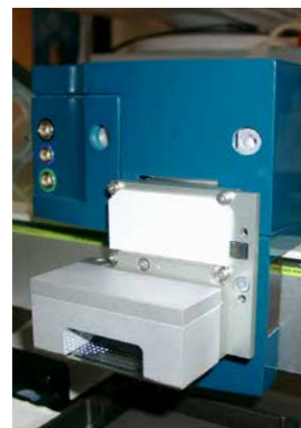
A700-900,901 Nano-Plotter head with holder for pin tool contact dispensers. Pin tools require a spring-loaded slide deck.
