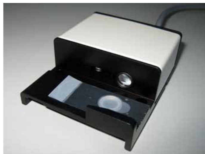
A070-012 Stroboscope (spare, top) with LED, mirror, camera, and cable. Bottom: image processing of the stroboscope droplet pattern. Valid pixels (green) are used for droplet volume calculation.
