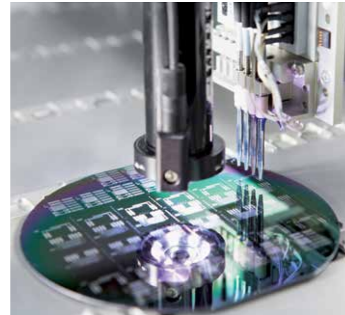
A070-017,023 Video microscope with ring light above microstructured wafer. Note that the microscope holder must be changed when also using the target visualization camera (below) or a two-row pipette holder (A072-006).
