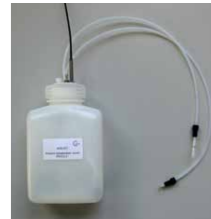
A072-130,140 Pressure compensation vessel, complete (tubes and filters not included) with two thick PTFE tubes (fluidic stage 2) connecting to two fluid distribution blocks
