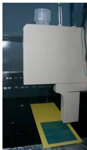
A010-400 Cartridge dispenser PEEK, printing arrays onto water-sensitive paper
