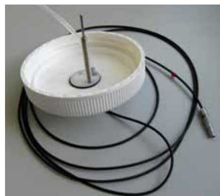
A072-226 Liquid level sensor in the cap of the waste bottle (sensor for pressure compensation bottle identical)
