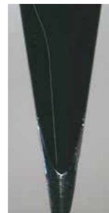
A070-403 Nano-Tip with sharpened tip (A040-404 and A040-504 similar)
