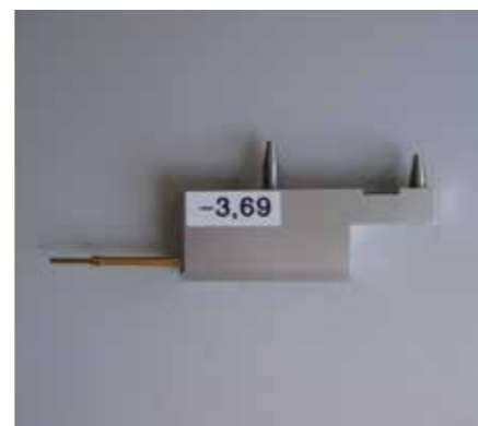
A072-223 Z-level sensor (NP 2.x). The switch point position relative to the pipette tip (printed number) is electronically stored in the device.
