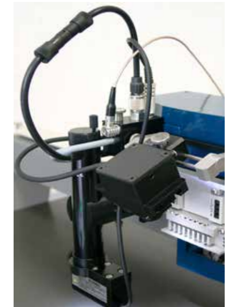
A070-073 Target visualisation camera, mounted together with video microscope (A070-023); both illuminated
