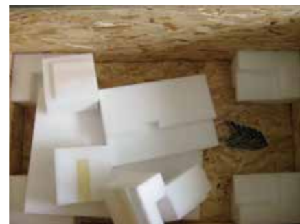
A076-004 Foam pads for NP 2.1/E crate (A076-003 similar), plus spring clips
