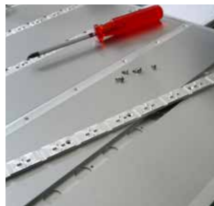
A070-064 Flipping the pins to obtain a flat deck
