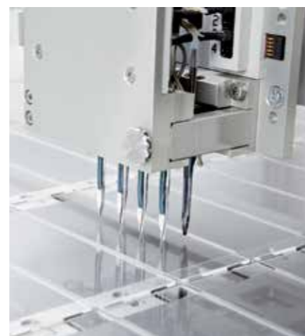
A072-006 Pipette holder (2x8) for Nano-Plotter (2.x), with 2 rows (first one swivels out) in 9 mm distance. Here, 8 J-type pipettes are mounted for spotting into 96-well plates.
