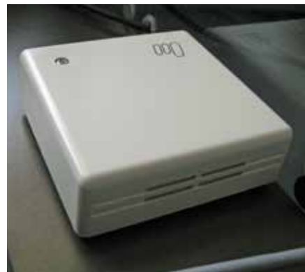
A072-016 Humidity sensor of the humidifying system
