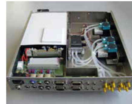
A072-296 Slide-in electronics module (NP 2.1; A072-230 similar); pumps and valves on the right
