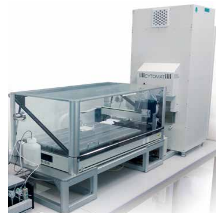
A070-043,048 Cytomat plate handler, connected to an NP 2.1/E via the adapter kit. This includes a stand on which the Nano-Plotter rests.
