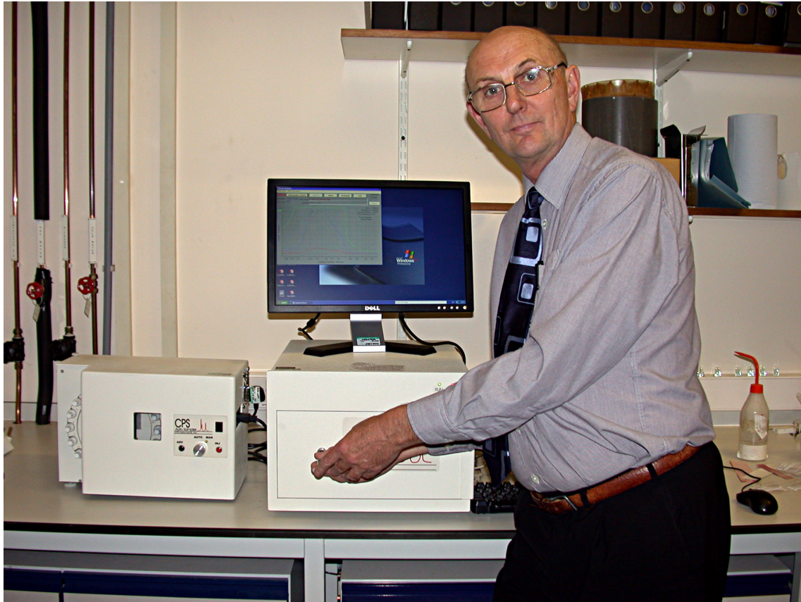
Dr. Bill Meredith making a sample injection on Intertek MSG's new CPS Disc Centrifuge. An autosampler was also purchased to enable fully unattended automatic injection of multiple samples and standards.
