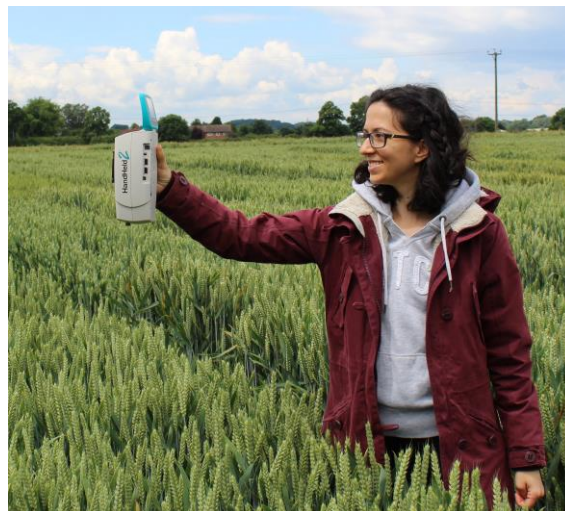
An ASD FieldSpec Handheld 2 portable spectroradiometer used to monitor differences in wheat crops
