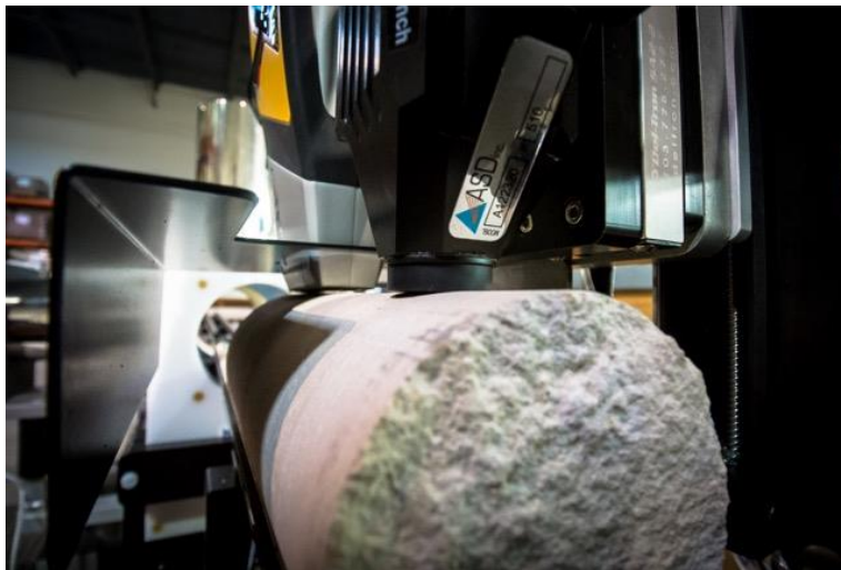
The ASD TerraSpec 4 making a measurement on a rock core in the Geotek MSCL system
