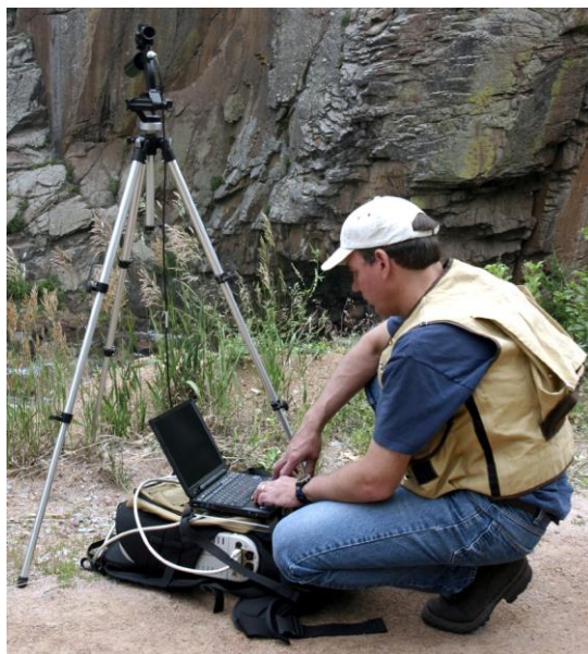
FieldSpec being used for rock mineral analysis
