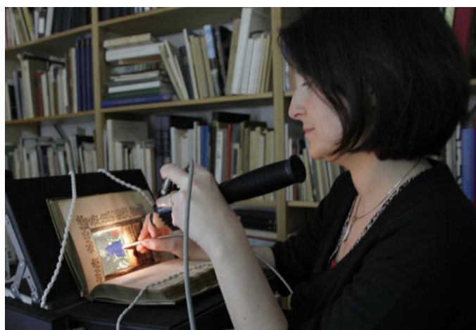
Dr Paola Ricciardi uses the ASD FieldSpec 4 spectroradiometer at the Fitzwilliam Museum, Cambridge
