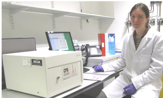
NPL's Nia Bell with the CPS disk centrifuge system for nanoparticle size characterisation.
